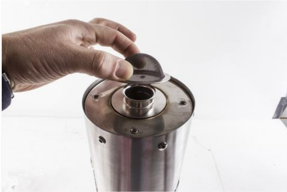
3: Insert the Spark Arrestor overtop of the Quiet Core.
